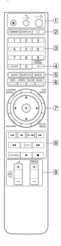
Number 5, AUDIO, PROG+, and buttons have a tactile dot. Use the tactile dot as a reference when operating the player.
